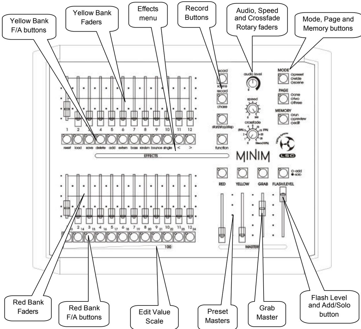
The front panel of the **MINIM** can be divided up into two areas:
